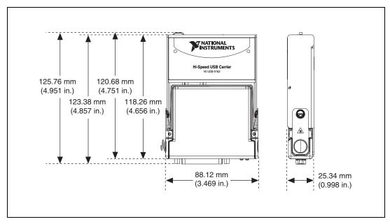
Figure 3. NI USB-9472 (D-SUB) Device in Millimeters (Inches)
